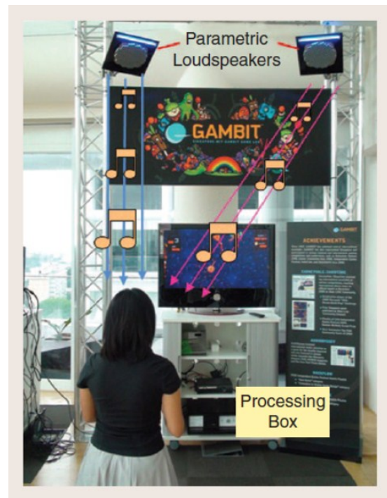
A pair of parametric loudspeakers installed in a gaming booth. Picture extracted from [2].
