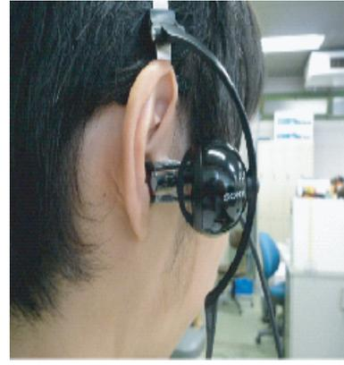
Fig. 4. Head-mounted ANC system.
