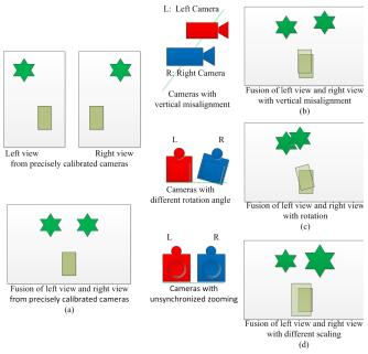
Fig. 1 Geometrical camera distortions [10].
