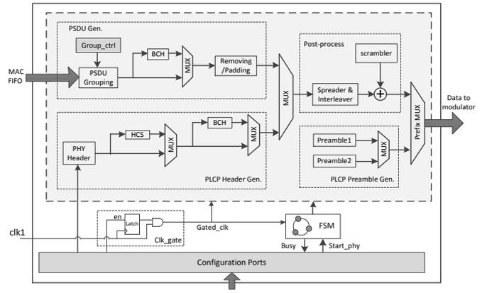
Fig. 3. Block diagram of PHY Module
