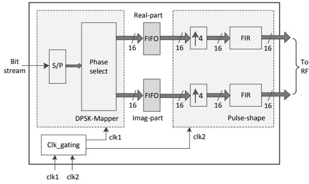
Fig. 5. Block diagram of DPSK Modulator
