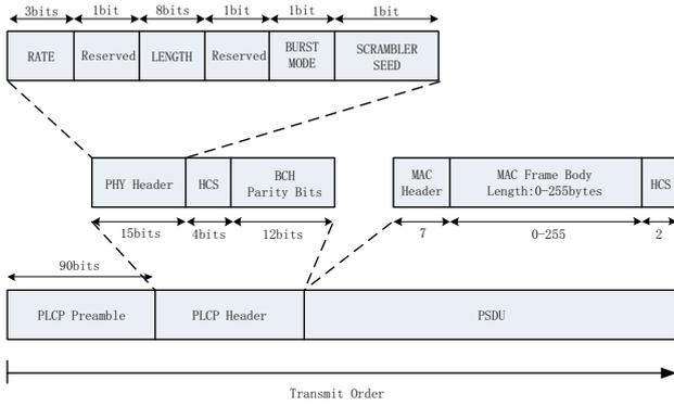
Fig. 2. IEEE 802.15.6 PPDU structure
