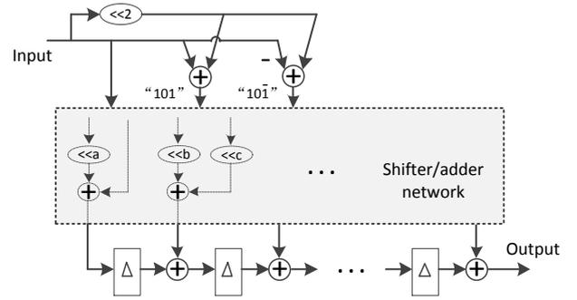
Fig. 6. CSD-based FIR filter
