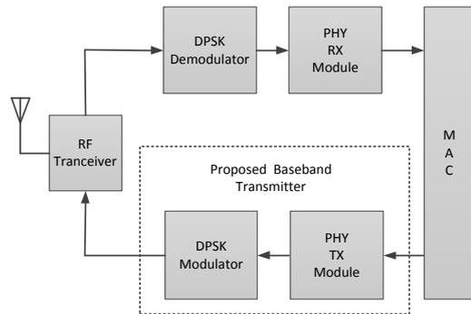
Fig. 1. Block diagram of a complete WBAN radio transceiver
