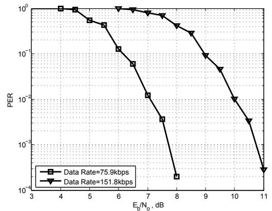
Fig. 7. Performance of baseband PHY system under MICS Band
