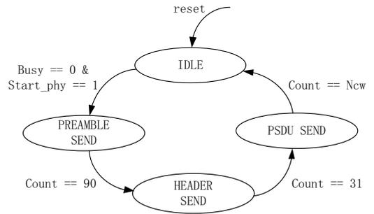
Fig. 4. PHY Module control machine
