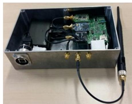
Fig. 10. BentoBox: Hybrid communication sensor node.
