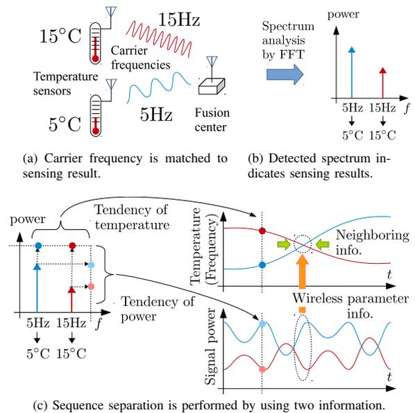
Fig. 1. The operation principle of PhyC-SN.
