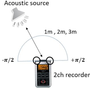
Fig. 3. Positional relationship between acoustic source and stereo microphone.
