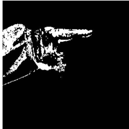
Fig. 3. Result of the GMM foreground segmentation applied to Fig. 1.
