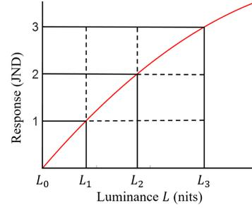
Fig. 1. Illustration of the luminance to HVS response mapping function  $r(L)$ .
