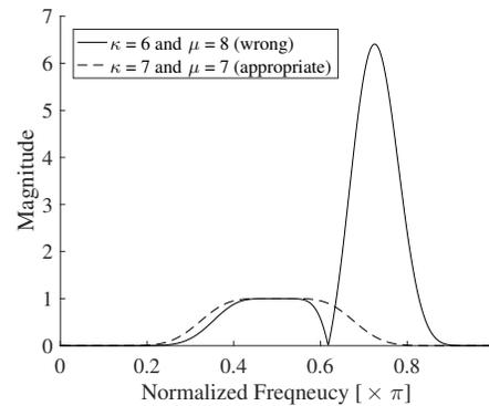
Fig. 1. The frequency response of band-pass MF FIR digital filters with wrong parameters and appropriate parameters
