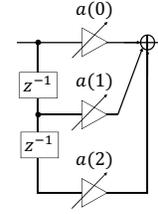
Fig. 2. The structure for the 2nd order variable FIR digital filters
