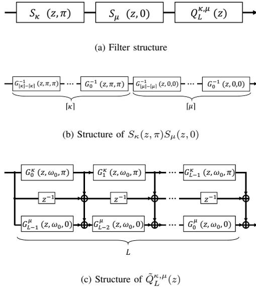
Fig. 3. The proposed structure for linear phase frequency-selective variable MF FIR digital filters
