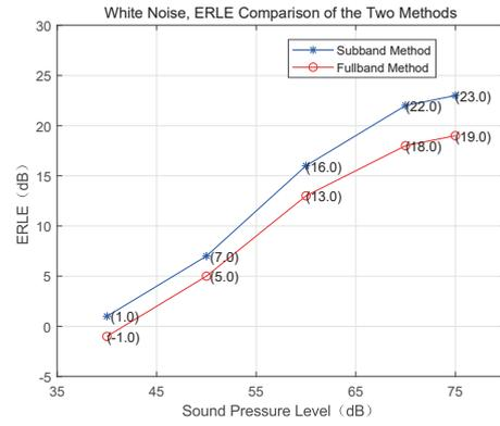
Fig. 11. Signal  $x$  is a white noise signal, ERLE values at different SPLs.
