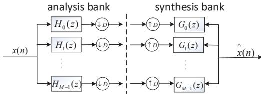
Fig. 4. Analysis and synthesis branch of a  $M$ -channel filter bank with subbands decimated by  $D$ .
