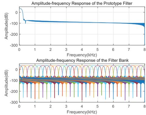
Fig. 6. Amplitude-frequency response of the prototype filter and filter bank.
