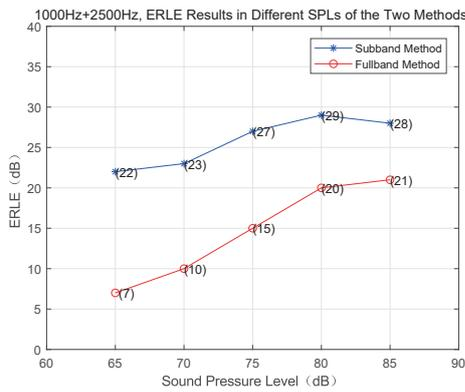
Fig. 13. Signal  $x$  is a 1000Hz+2500Hz signal, ERLE values at different SPLs.
