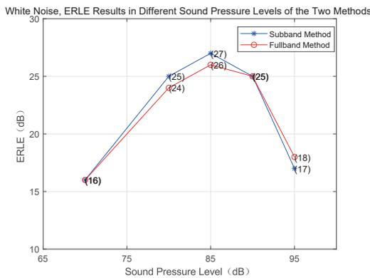
Fig. 14. Signal  $x$  is a white noise signal, ERLE values at different SPLs.
