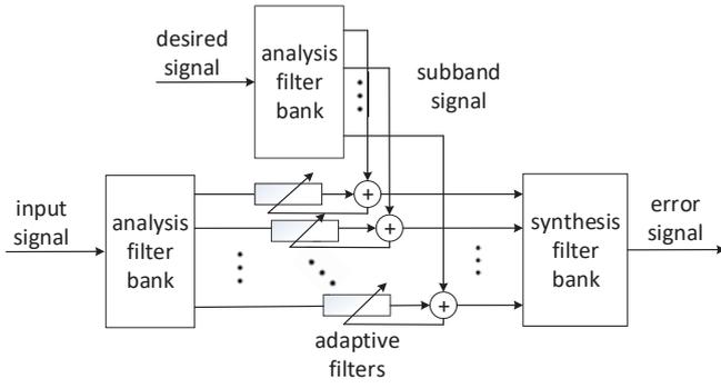
Fig. 3. Set-up of the subband echo cancellation.
