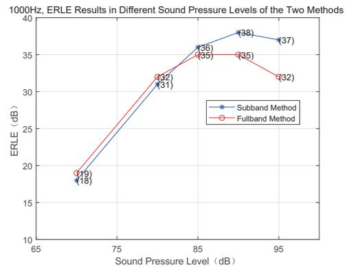
Fig. 12. Signal  $x$  is a 1000Hz single-frequency signal, ERLE values at different SPLs.
