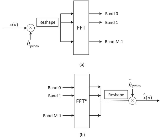
Fig. 5. The subband analysis (a) and synthesis (b) using DFT-modulated polyphase filter bank.
