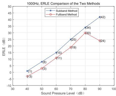
Fig. 10. Signal  $x$  is a 1000Hz single-frequency signal, ERLE values at different SPLs.
