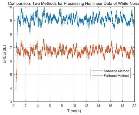
Fig. 9. Signal  $x$  is a white noise signal, ERLE comparison.
