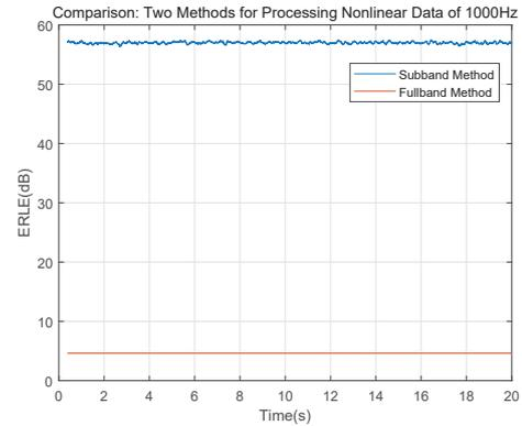
Fig. 8. Signal  $x$  is a 1000Hz single-frequency signal, ERLE comparison.
