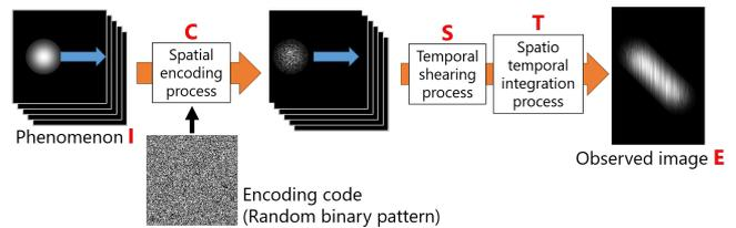
Fig. 1. Formulation of image acquisition process.
