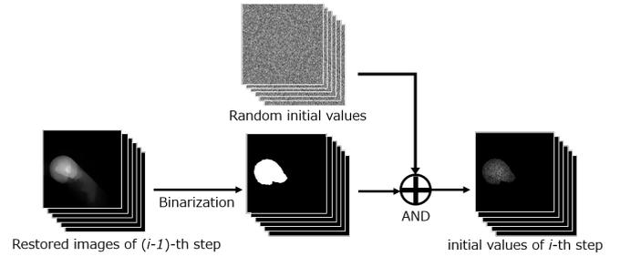
Fig. 3. Scheme of estimating initial values of  $i$ -th ( $= 2, 3, \dots, N$ ) step in N-CUP method.
