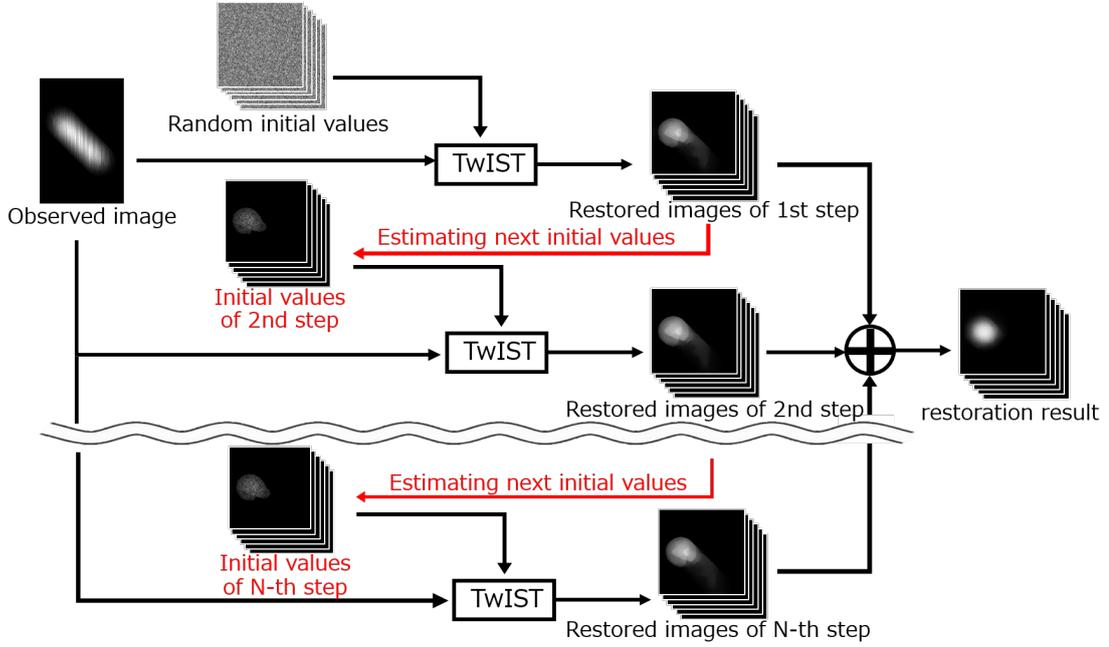
Fig. 2. Overview of the restoration process in N-CUP method.
