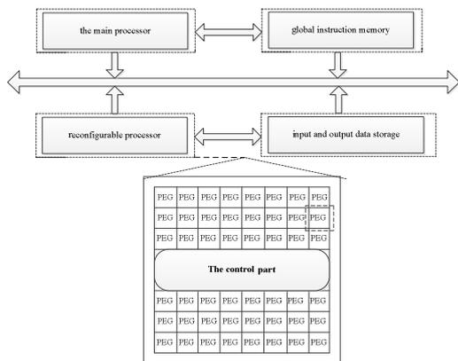
Fig. 1 Single processing element cluster
