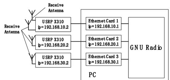
Fig. 3 Cooperative Spectrum Sensing Hardware System
