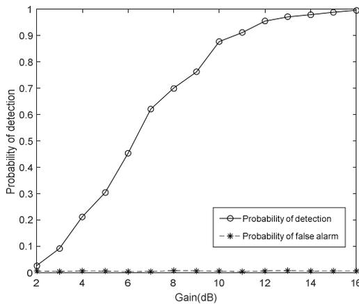
Fig. 8 Probability of detection of the hardware sensing system
