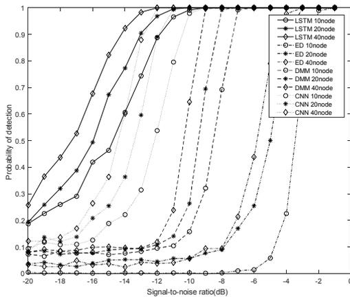
Fig.6.  $P_d$  of four algorithms under different SNR
