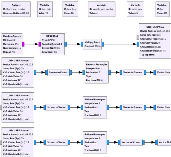
Fig.4 USRP transceiver flow diagram built in GRC
