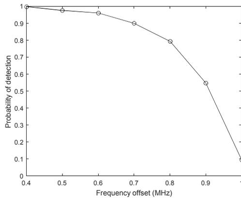
Fig.9. Anti-frequency offset performance of the hardware sensing system
