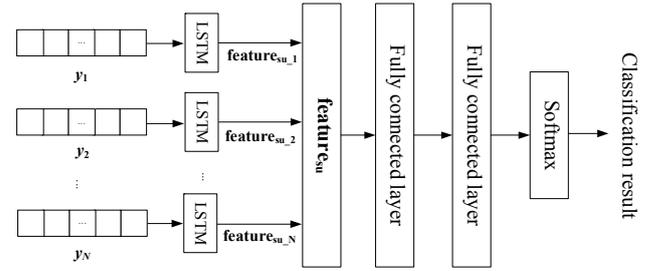
Fig. 2 Cooperative Spectrum Sensing Model Based on LSTM
