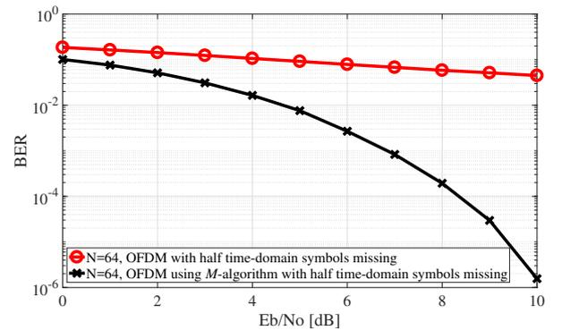
Fig. 2. BER performance of the OFDM system with BPSK modulation using  $M$ -algorithm compared to that of the conventional OFDM system when half time-domain symbols are missing in the AWGN channel.
