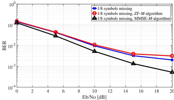
Fig. 3. BER performance of the OFDM system for BPSK modulation using  $M$ -algorithm with ZF or MMSE compared of that of the conventional OFDM system when 1/8 time-domain symbols are missing in the WLAN channel model.
