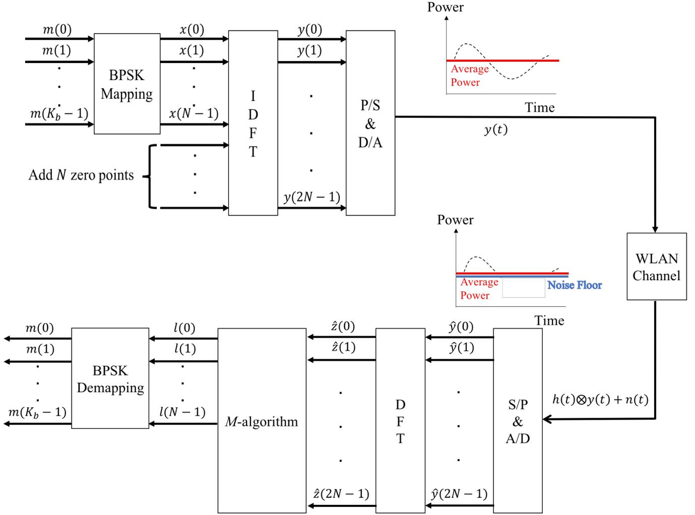
Fig. 1. Structure of OFDM system with BPSK modulation using  $M$ -algorithm when the partial time-domain symbols are missing.
