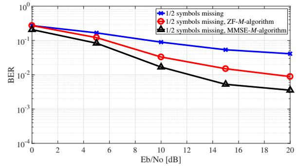
Fig. 5. BER performance of the OFDM system for BPSK modulation using  $M$ -algorithm with ZF or MMSE compared of that of the conventional OFDM system when 1/2 time-domain symbols are missing in the WLAN channel model.
