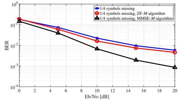
Fig. 4. BER performance of the OFDM system for BPSK modulation using  $M$ -algorithm with ZF or MMSE compared of that of the conventional OFDM system when 1/4 time-domain symbols are missing in the WLAN channel model.
