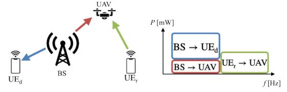
(a) Packets flow and allocation of bandwidth, power in STEP1
