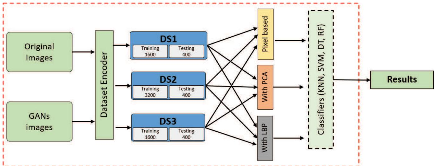
Fig. 4: The general framework of the experiments. We created three sets out of the entire dataset: DS1, DS2, and DS3. Each set is tested three times on four different ML classifiers.
