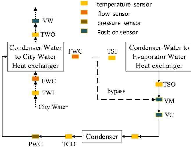
Fig. 5 Location of sensors on the condenser.
