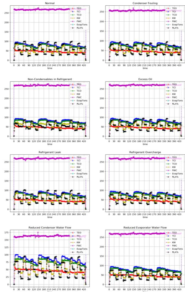
Fig. 6 Visualization of the 6-dimensional parameters in different fault conditions.
