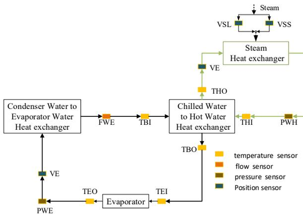
Fig. 4 Location of sensors on evaporator.
