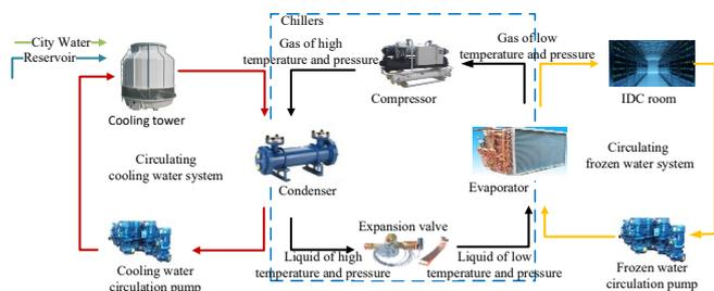
Fig. 1 Refrigeration system of Internet Data Center.
