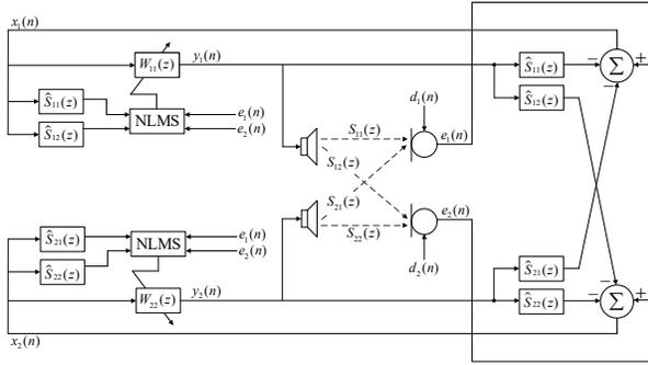
Fig. 2. Block diagram of the  $2 \times 2$  MCFBANC system without the cross-channel control filters.
