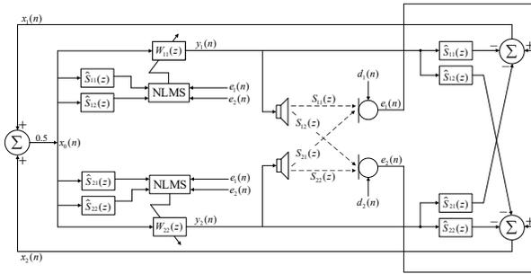
Fig. 3. Block diagram of the  $2 \times 2$  MCFBANC system with the mixed reference signal estimate.
