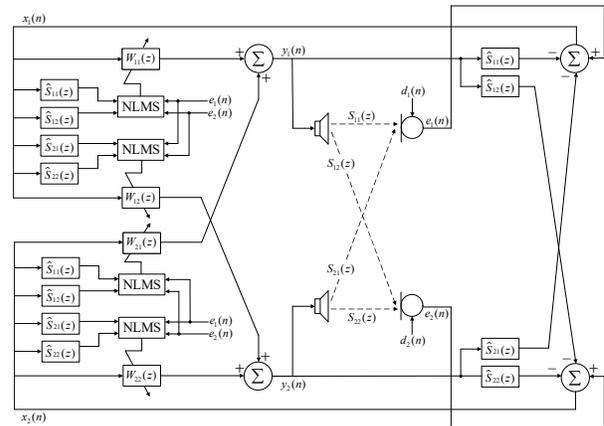
Fig. 1. Block diagram of the  $2 \times 2$  MCFBANC system with the cross-channel control filters.
