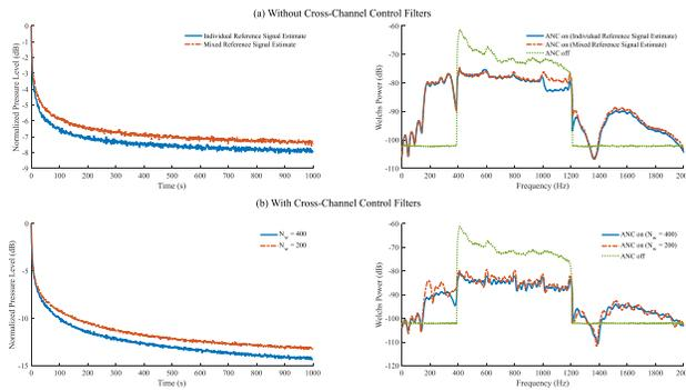
Fig. 10. MCFBANC system performance when the primary noise is a broadband noise.
