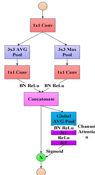
Fig.5 Downsampling unit network model.
