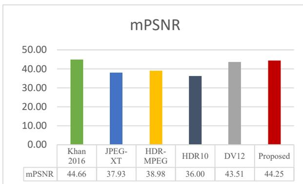
Fig. 5 HDR Peak Signal to Noise Ratio
