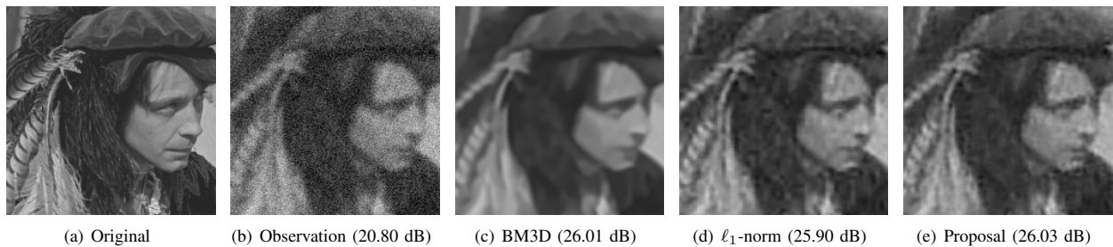
Fig. 8. Image denoising result when \sigma_w = 20 for "Man". (a) Original image, (b) Observation image (PSNR: 20.80 dB), (c) Restored image with BM3D (PSNR: 26.01 dB), (d) Restored image with the \ell_1 -norm regularization (PSNR: 25.90 dB), (e) Restored image with the proposed method (PSNR: 26.03 dB).
