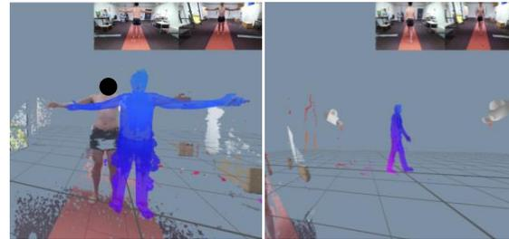
Fig. 3 “T” pose for skeleton fitting (left). Gait analysis using the dual Azure Kinect motion capture system (right).
