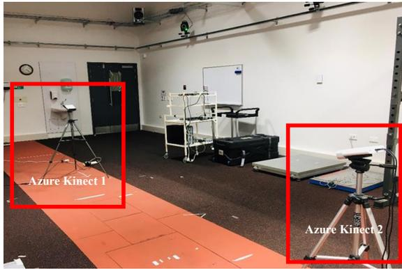
Fig. 1 Experimental setup for the dual Azure Kinect motion capture system
