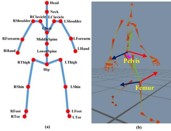
Fig. 4 Stick figure model obtained from the Azure Kinect in the iPi software (a). The definition of the pelvis and femur coordinate system (b).
