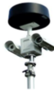
Fig.1 Surveillance system with sensor fused with radar at the top and camera at the bottom
