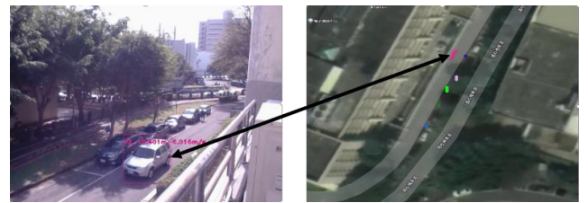
Fig. 26 Estimation of the speed of the object moving at 20 km/h (5.56m/s) by the proposed sensor fusion method.
