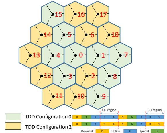
Fig. 1 Heterogeneous TDD slot configurations system.
