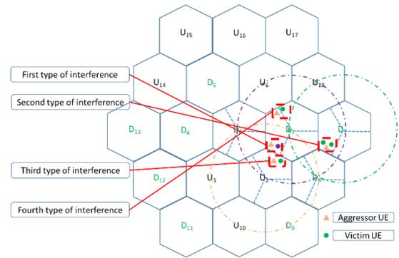
Fig. 3 Four types of UE-UE interference.
