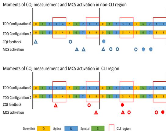
Fig. 6 Dual tracks of CQI feedback mechanism.
