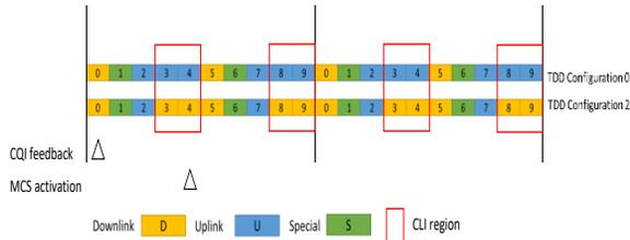
Fig. 5 Aggressor UE interferes with Victim UE in heterogeneous TDD system.
