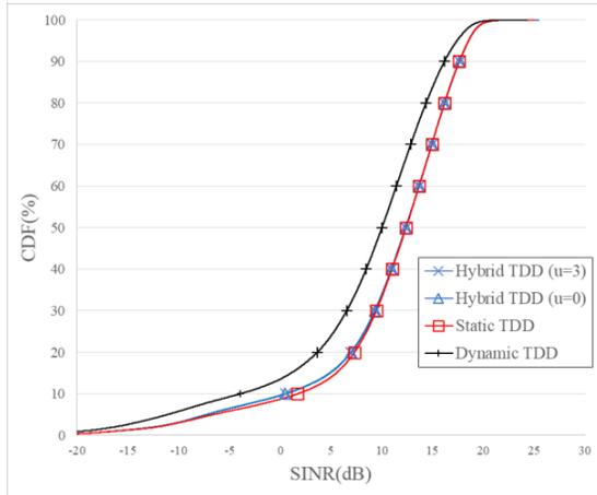
Fig. 8. UL SINR under different TDD schemes
