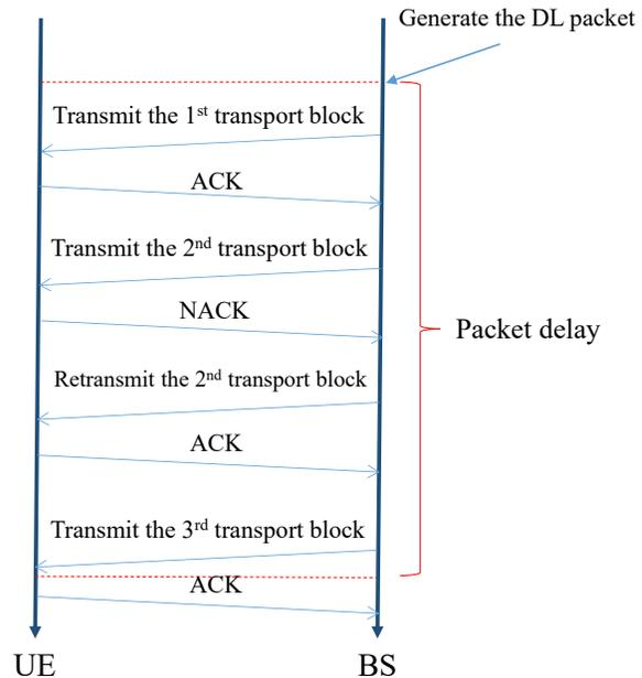
Fig. 2. Illustration for the packet delay
