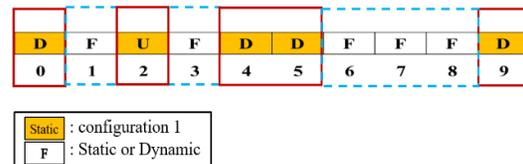
Fig. 3. Illustration for the frame structure for the proposed hybrid TDD system
