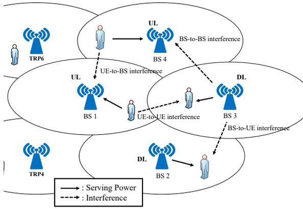
Fig. 1. Dynamic TDD interference scenario
