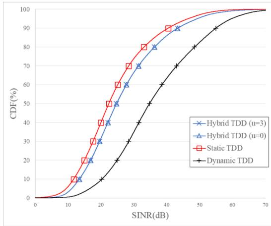
Fig. 7. DL SINR under different TDD schemes
