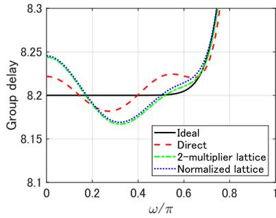
Fig. 2. Group delay characteristics of quantized all-pass fractional delay filters ( $D = 8.2$ ).
