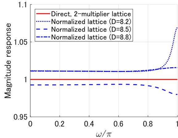
Fig. 5. Magnitude responses of quantized all-pass fractional delay filters.
