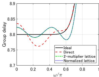
Fig. 4. Group delay characteristics of quantized all-pass fractional delay filters ( $D = 8.8$ ).
