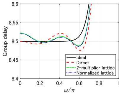
Fig. 3. Group delay characteristics of quantized all-pass fractional delay filters ( $D = 8.5$ ).
