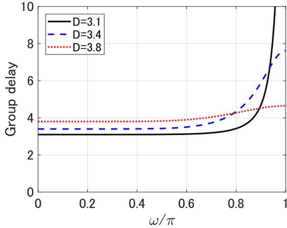
Fig. 1. Example of group delay characteristics of all-pass fractional delay filters.
