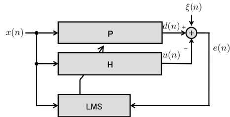
Fig. 1. Block diagram of the adaptive system.
