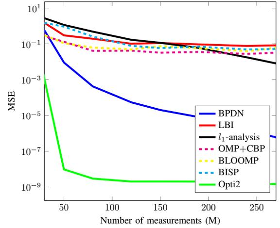
Fig. 2. Performance comparison of different reconstruction algorithms in terms of the MSE vs.  $M$ .
