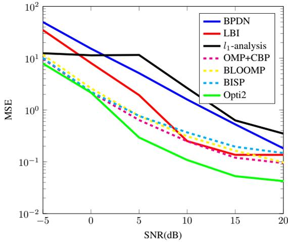
Fig. 1. Performance comparison of different reconstruction algorithms in terms of the MSE vs. SNR.
