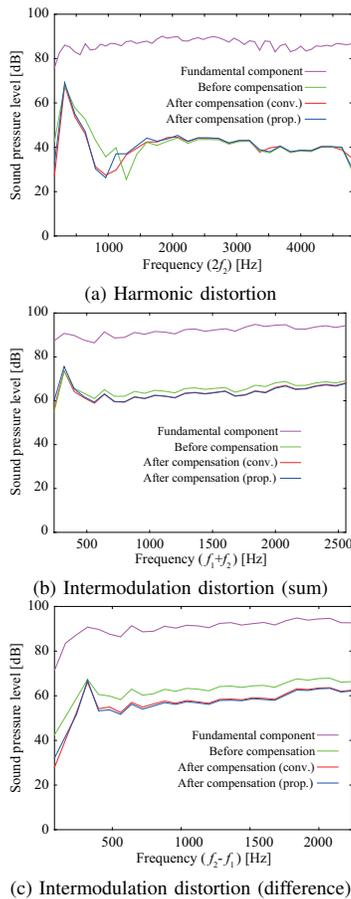
Fig. 7. Compensation results for second-order nonlinear distortion.
