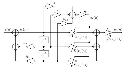
Fig. 1. Block diagram of second-order nonlinear IIR filter [11], [12].
