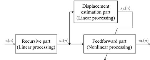
Fig. 2. Simplified block diagram of second-order nonlinear IIR filter [15].
