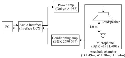
Fig. 6. Arrangement of measurement devices.
