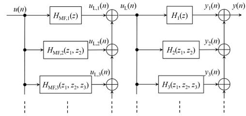
Fig. 3. Compensation model of second-order nonlinear IIR filter.
