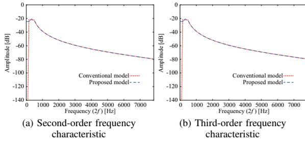
Fig. 4. Diagonal elements of multidimensional frequency characteristics.
