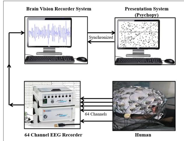
Fig. 2: EEG Acquisition Apparatus
