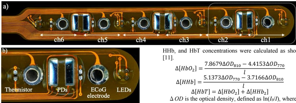
Fig. 1 Microphotograph of the multimodality probe. (a) Probe head with 6 channels for ECoG, NIRS, and thermistor signals. White arrows show the distribution of ch1–ch6. (b) Enlarged view of the white dotted area.
