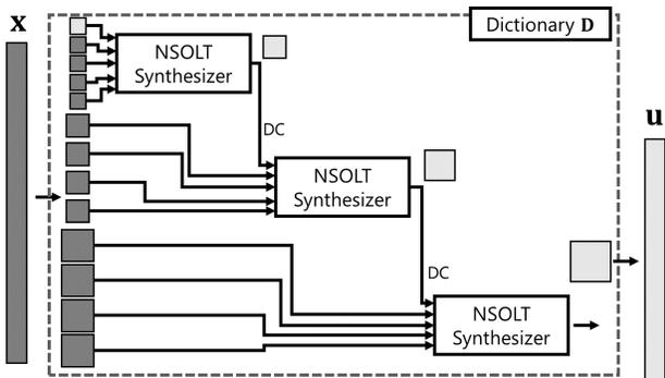
Fig. 3. A 3-level tree structure of multiscale synthesis NSOLT [15]
