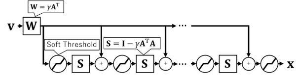
Fig. 1. Architecture of LISTA, where ISTA's loop is unrolled. The matrices  $\mathbf{W}$  and  $\mathbf{S}$ , are learned, so as to minimize the approximation error of the optimal sparse codes on a given dataset [8].
