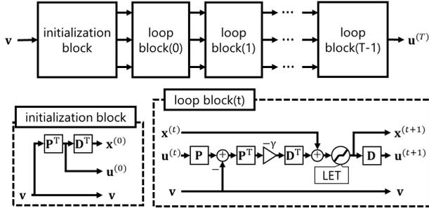
Fig. 2. Architecture of proposed loop unrolling network, where  $\mathbf{D}$  is a synthesis dictionary and  $\mathbf{P}$  is a measurement process.  $\mathbf{D}^T$  is the adjoint of  $\mathbf{D}$  and has the role of analyzer. Note that  $\mathbf{D}$  and  $\mathbf{D}^T$  are independently trained so that the backpropagation is available.
