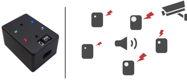
Fig. 1: Sound-to-light conversion device Blinky (left) and acoustic sensing framework using Blinky and single video camera (right).
