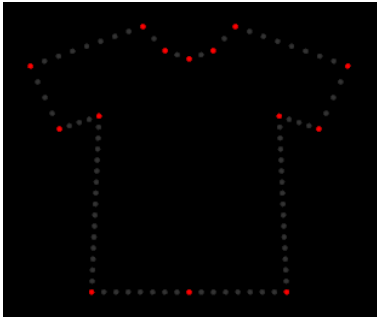
Fig. 3 The inserted nodes and the detected feature points form the garment boundary. Red points present feature points and gray points are the inserted points.
