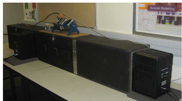
Figure 3. The implemented ANC system in the acoustic duct
