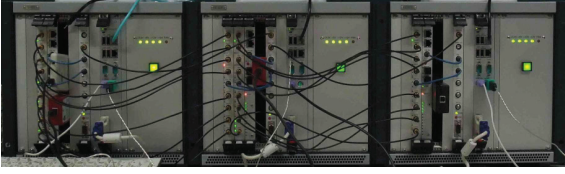
Fig. 1. Channel emulator (centre) together with TX and RX systems.
