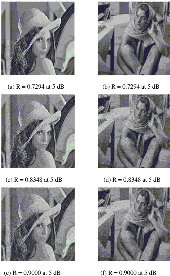
Fig. 5 Comparison of the transmitted images for three rates at the same SNR.
