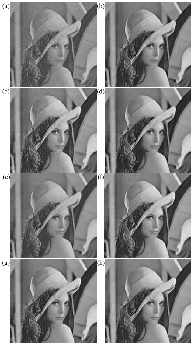
Fig.3. Subjective quality comparison of denoised images different denoising methods. (a) Noisy image, PSNR =20.17 dB, SSIM = 0.600; (b) BLS-GSM, PSNR = 31.70dB, SSIM = 0.921; (c) Curvelet, PSNR =30.63 dB, SSIM = 0.895; (d) Contourlet, PSNR = 31.06dB, SSIM = 0.912 ; (e) NLM, PSNR = 30.44dB, SSIM = 0.910; (f) SA, PSNR = 31.62dB, SSIM = 0.920 ; (g) BM3D, PSNR = 32.06dB, SSIM = 0.926; (h) Proposed, PSNR = 31.53dB, SSIM = 0.922.
