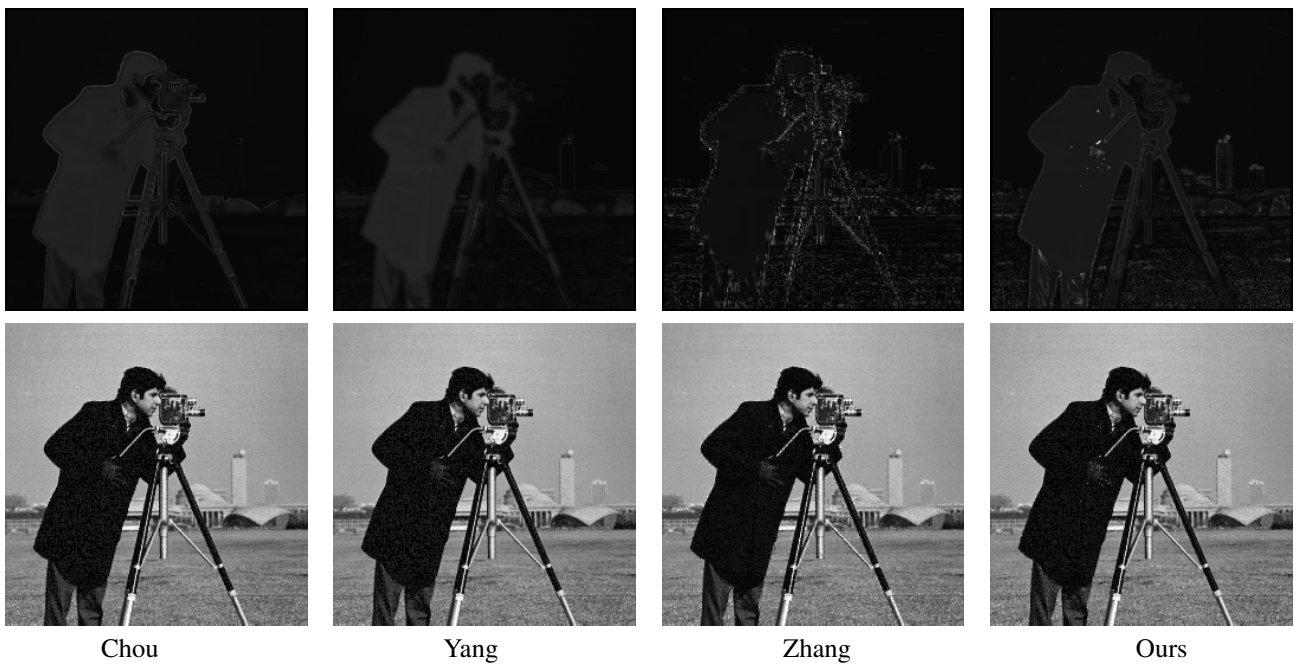
Fig. 5: Performance comparison of JND estimation methods on the test image cameraman. The top row shows JND masks and the bottom row the JND guided noisy images (under the same energy of noise level with MSE = 63.35 ). Our method gives the most comfortable visual experience, because our method adds most noise to the grassland in the image where more noise can be concealed.
