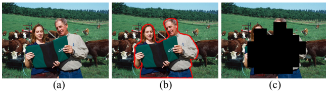
Fig.5. Another example of JPEG image forgery detection: (a) composite JPEG image;(b) ground truth of (a), the tampered region are bounded by the red contour;(c) detected tampered region by the proposed method.
