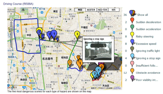
Fig. 16. Interface summarizes hazardous situations on a driving map.
