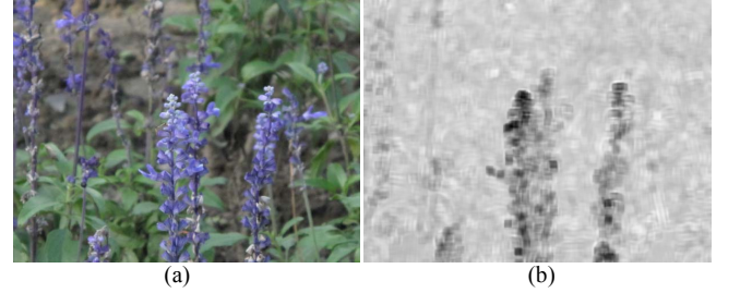
Fig.2. The test image and its saliency map. (a) A color image of sized 1104 \times 828 , and (b) the saliency map. The light-gray pixel and the dark-gray pixel correspond to big blurriness and small blurriness, respectively.
