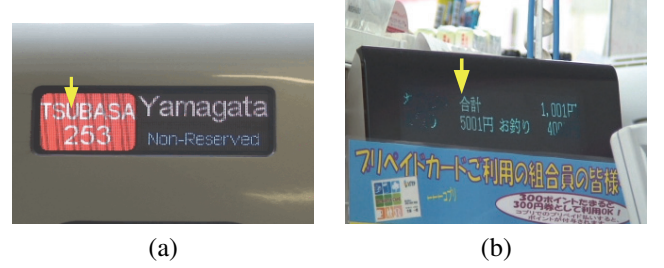
Fig. 1. Streaks arising on an LED monitor (a) and a VFD monitor (b). The arrows point to manually selected sampling pixels to detect the blinking interval.
