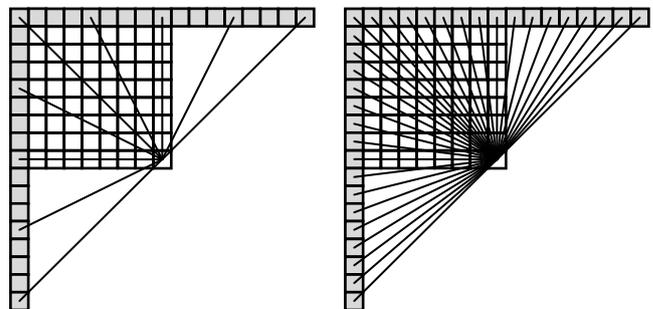
Fig. 1 Intra prediction directions of H.264/AVC (left) and HEVC (right).
