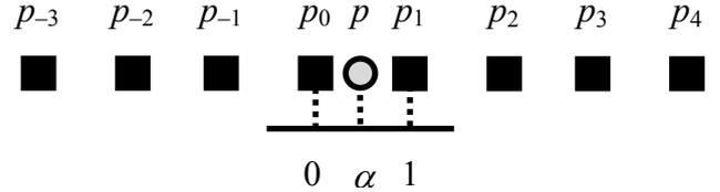
Fig. 3 Integer pixel positions (black squares) and an interpolated pixel (a shadowed circle) in DCT-IF.
