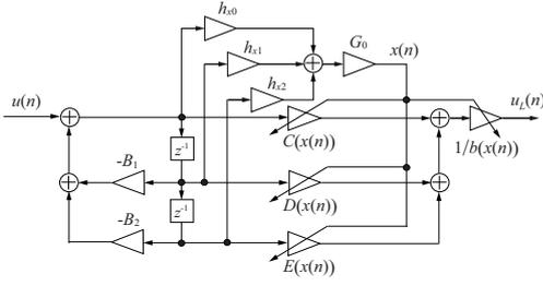
Fig. 2. Block diagram of the 2nd-order nonlinear IIR filter.
