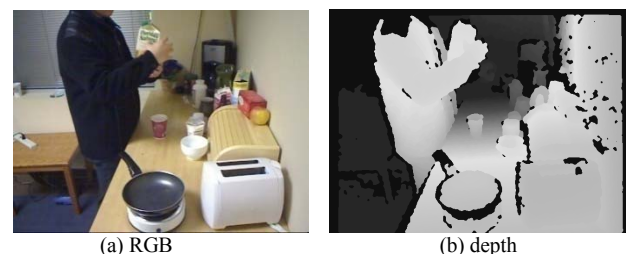
Fig. 2. Synchronized depth and RGB images. Image (b) is a depth map of (a), with lighter shades closer to the camera.
