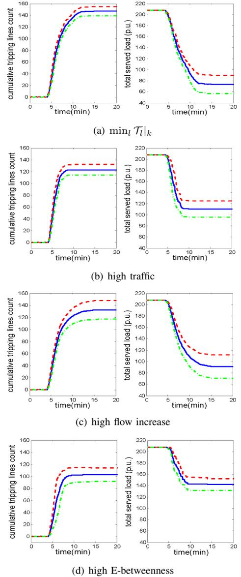
Fig. 5. The cascading process in the IEEE-300 system triggered by tripping one of the most critical lines identified the four vulnerability measures as indicated below each sub-figure: the mean value of line outages and load served (blue); the range of half standard deviations (red and green).
