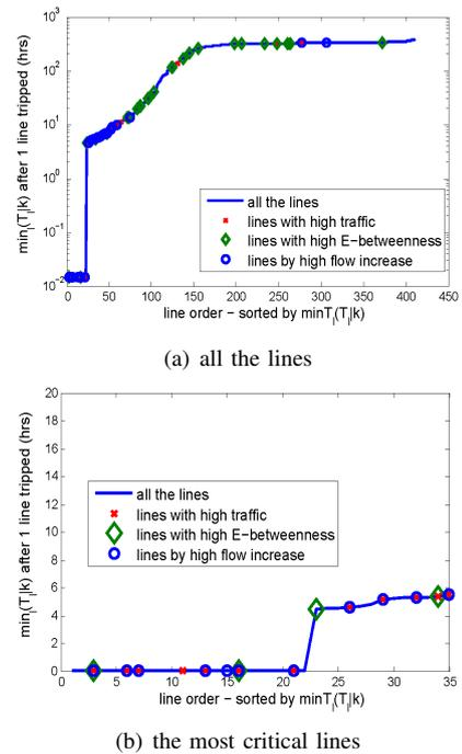
Fig. 3. The minimum safety time after 1 line tripped: the IEEE-300 system
