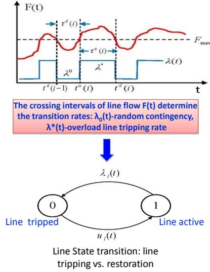
Fig. 1. The flow process and the line state transition
