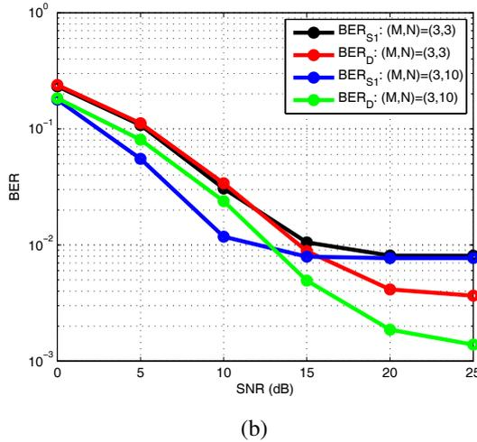
Fig. 3. Performances of multi-relay two-way network with multiuser interference. (a) BER of the system with the number of relays:  $N = 3$  and  $N = 5$ . (b) BER of the system with the number of relays:  $N = 3$  and  $N = 10$ .
