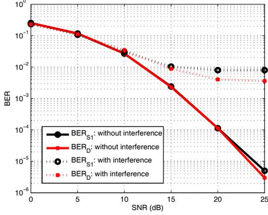
Fig. 2. Comparison of the proposed algorithm to an interference-free case.
