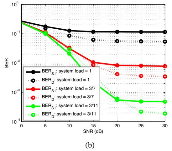
Fig. 4. Performance of multi-relay two-way network with multiuser interference. (a) BER of the system with the number of users:  $M = 3$ ,  $M = 6$  and  $M = 9$ . (b) BER of the system with the length of spreading sequence:  $K = 3$ ,  $K = 7$  and  $K = 11$ .
