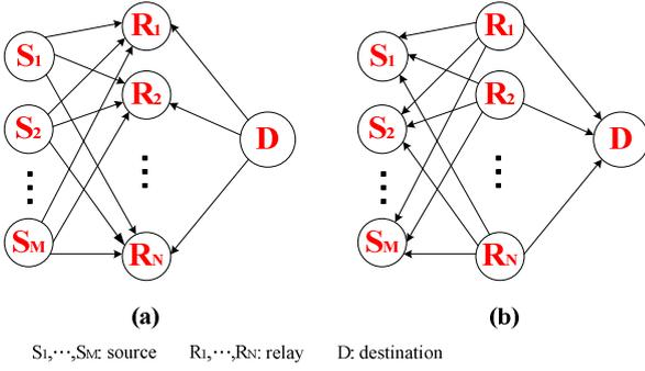
Fig. 1. A multi-source, multi-relay and single destination network. (a) 1st time slot. (b) 2nd time slot.
