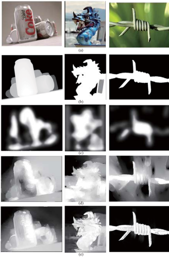
Fig. 6. Visual comparison of extracted depth maps due to camera defocus: (a) the original image, (b) the ground-truth depth map, (c) the depth map result based on the deblur model in [5], (d) the depth map result based on the defocus magnification algorithm in [4], and (e) the depth map result of the proposed algorithm.
